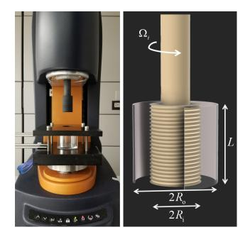
Figure 2: Image of the experimental Taylor-Couette setup, attached to a stresscontrolled rheometer on the left, and a schematic of the setup, on the right.
